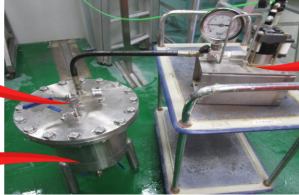
5 ATM testing equipment
